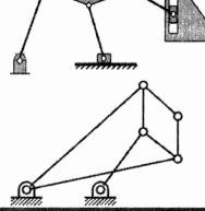
Q.3(A) Locate all the instantaneous centres for a four-bar mechanism as shown in Figure. The lengths of various links are: AD = 125 mm; AB = 62.5 mm; BC = CD = 75 mm. If the link A B rotates at a uniform speed of 10 r.p.m. in the clockwise direction, find the angular velocity of the links BC and CD.
